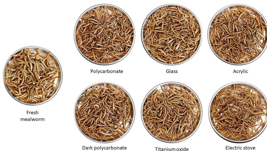
FIGURE 5 Visual comparison of the yellow mealworm ( Tenebrio molitor L.) drying process using different types of covers of solar dryers.
