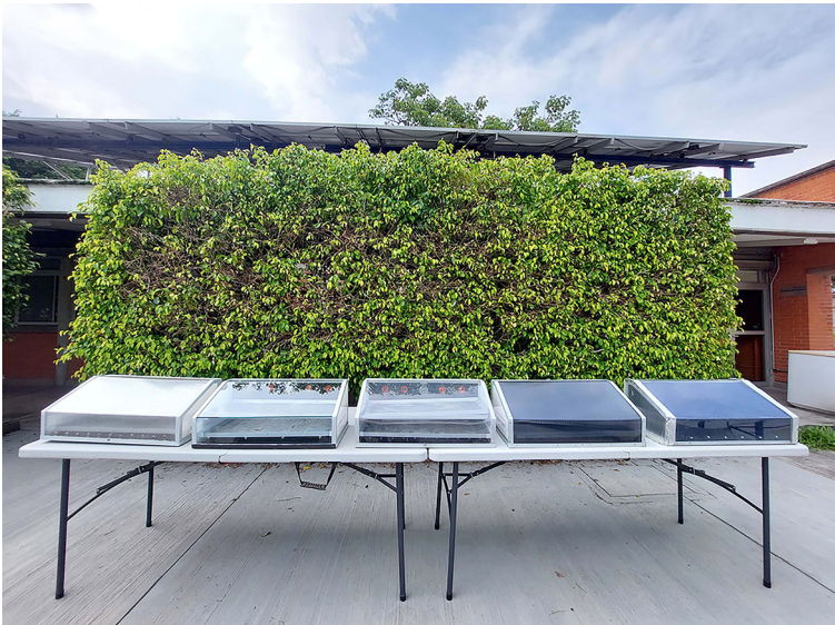
FIGURE 1 Different types of covers of solar dryers used in the drying process of Tenebrio molitor L. From left to right: polycarbonate, glass, acrylic, dark polycarbonate and aluminium with titanium oxide.
