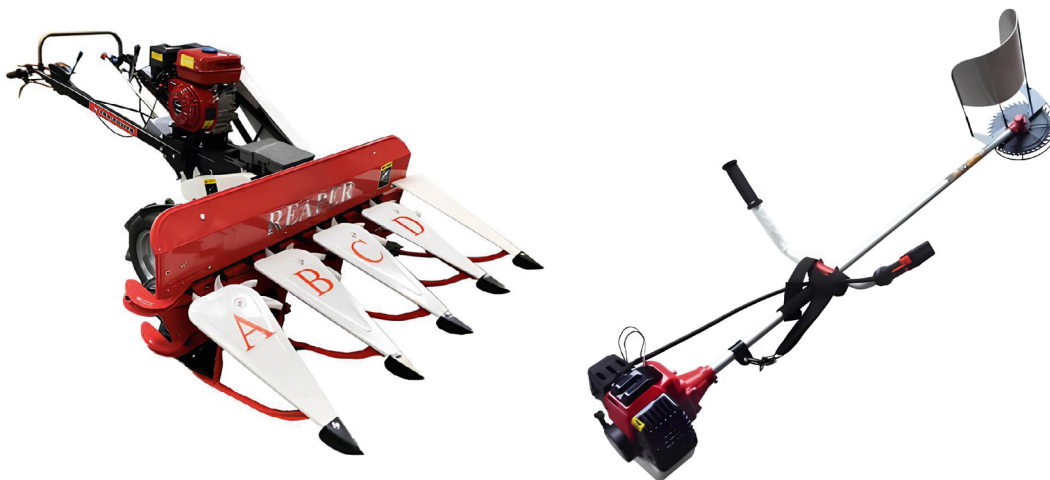
Figure 1. (Left) Reaper-harvester (source: shellermachine.com); (right) mini harvester (source: farmpays.com).
