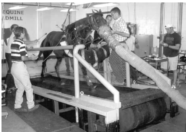
FIG. 2 The Thoroughbred horse ( Equus caballus ) running on a high-speed equine treadmill. Through thousands of years of selective breeding, this animal is one of the top athletes in the world, achieving maximal \dot{V}O_2 values 2 exceeding 200 \text{ ml min}^{-1} \text{ kg}^{-1} . The bias-flow system seen here enables collection of respired gases and high-fidelity resolution of \dot{V}O_2 kinetics
