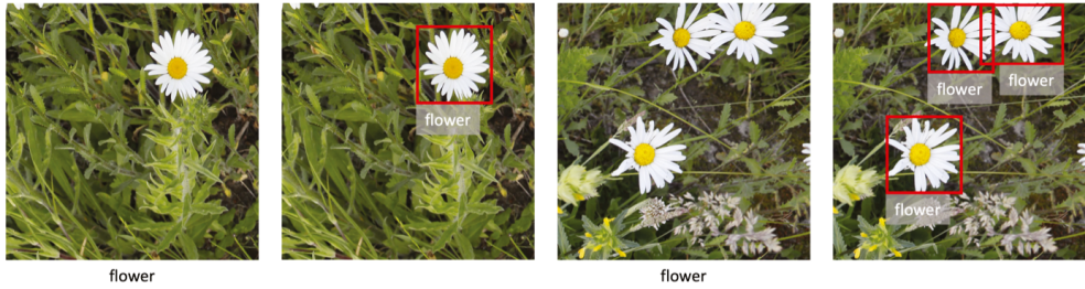
FIGURE 14.2 Image recognition and object detection comparison. Image recognition (first and third) labels the entire image, while object detection (second and fourth) localizes objects in an image by drawing bounding boxes around them and then labels them accordingly. Photos are crops from EWD images (Schouten et al. , 2024)
