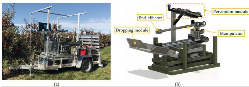
Figure 5. A photograph (a) and 3-dimensional sketch (b) of the robotic apple harvesting system integrated with the active laser-camera scanning (ALACS) unit.
