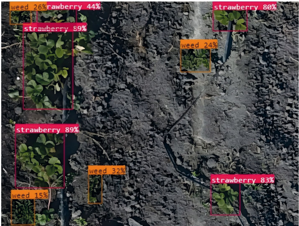
Figure 4. Detected strawberries in pink bounding boxes with weeds in orange bounding boxes.
