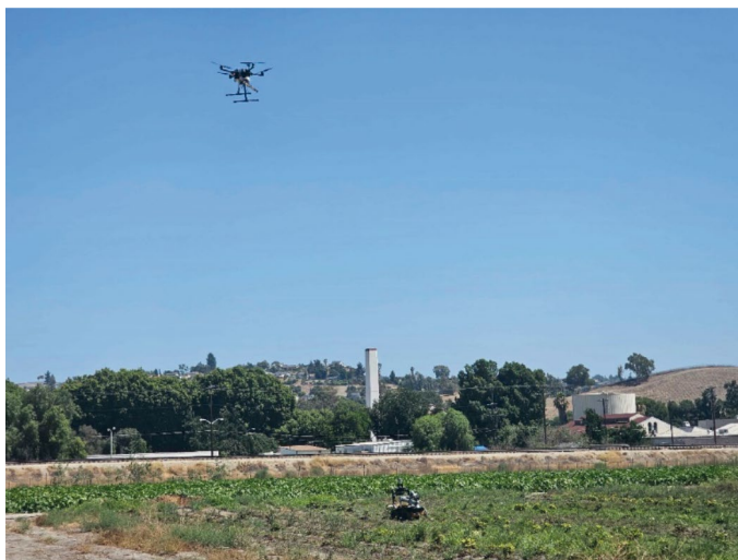
Figure 3. Experimental testing of the UAV-UGV collaboration for weed detection and removal.
