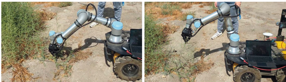
Figure 5. Extraction and disposal of a weed by the UGV.
