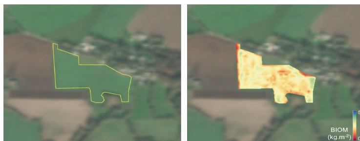
Figure 7. Example of a biomass map calculated using the developed methodology for a phacelia field. Calculated from a Sentinel2 image acquired on 22 November. (Left) The true colour image with the field contour in yellow; (Right) The fresh biomass map ( \text{kg}/\text{m}^2 ).
