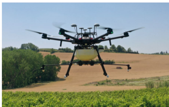
Figure 1. The UASS used for experimental purposes. The UASS consisted in the UAV Matrice 600 Pro equipped with a customized spray system.
