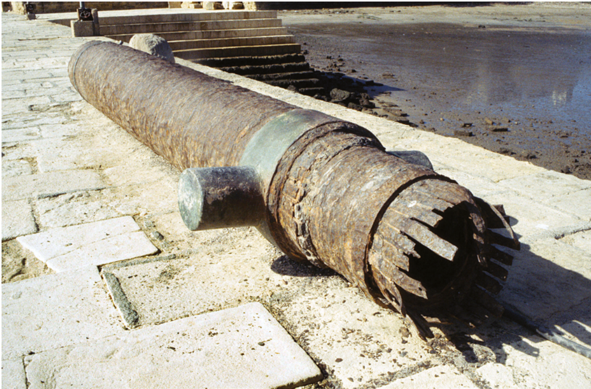
PLATE 2.3 Remains of the reinforce of a cannon, now laid abandoned on the jetty of the fort of Diu, seen from the exploded end of the chase. The structure of the cannon with laminated strips of steel is exposed at the point of explosion.
