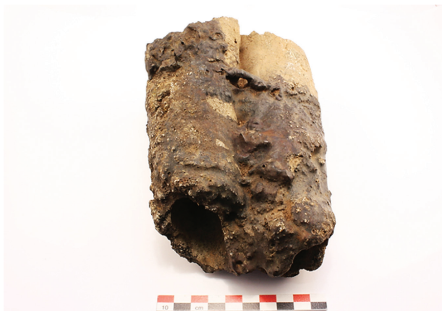
FIGURE 5.8 A double fused tuyeres from Veza B site
