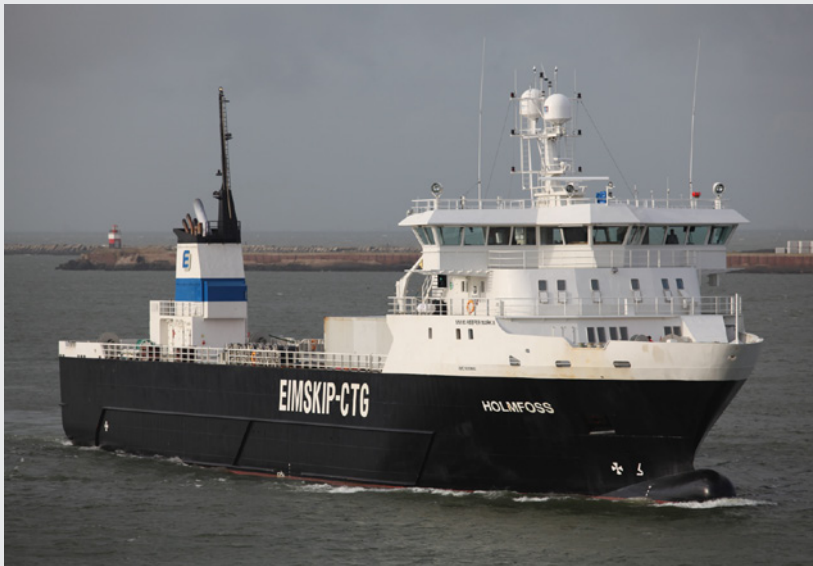
FIGURE 21 Small reefers like the Holmfoss connect Norway's fishing ports and Murmansk to the UK and the Continent. This vessel was delivered in 2008 and can handle different temperatures in its five holds. Eighty metres long, it can carry 28 FEU containers, with reefer plugs, and is rated to operate in one metre thick ice
