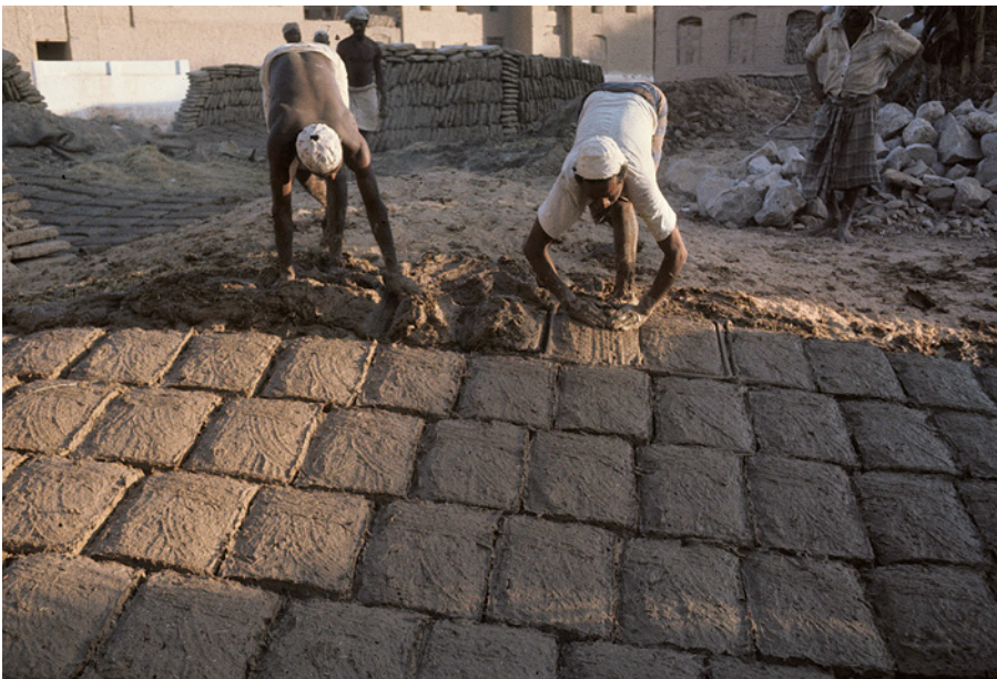
FIGURE 7.10 Mud bricks molds CREDITS: CHRISTIAN DARLES.
