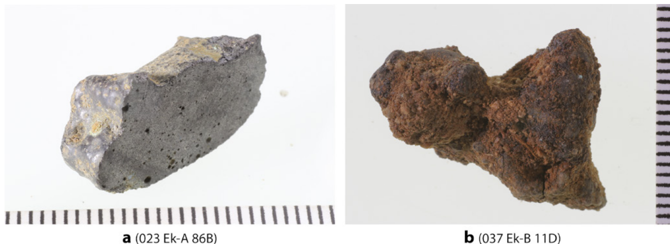
FIGURE 16.9 Essouk copper slag (only 'a' has been sectioned) (both sample and context number are provided here; see App. I for descriptions of examples shown here).
