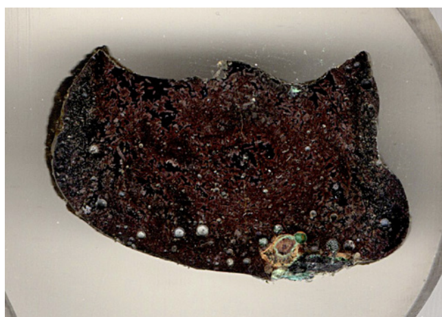
FIGURE 16.10 Polished block of copper slag sample Ek-A 86B (023). The orientation of the sample (upper or lower surface) is uncertain, but it does show a tap flow pattern. Width of cut sample is ca 2 cm.
