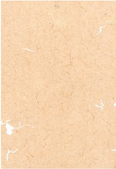
Fig. 136: Indian wove paper with visible undissolved fibres
