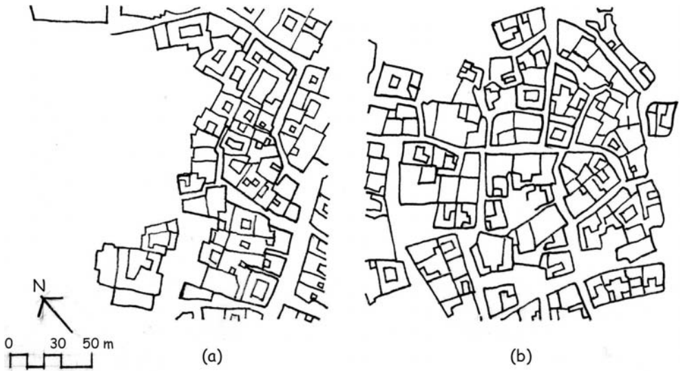
Fig. 1. Compact urban tissue resulting from abutting one structure against its neighboring structures. This was the predominant traditional pattern in the Islamic world. Two examples, drawn to the same scale, are illustrated here: On the left (a) is a partial plan from Sidi Bou Sa'id located on the Mediterranean in northern Tunisia. On the right (b) is a partial plan from Dar'iyah near Riyadh, Saudi Arabia. After sources from the author.
